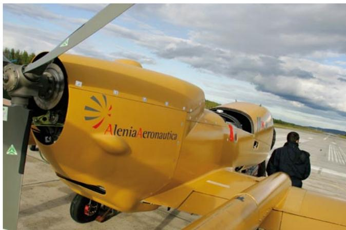
UAV SKY-Y during flight test at Vidsel test range.
