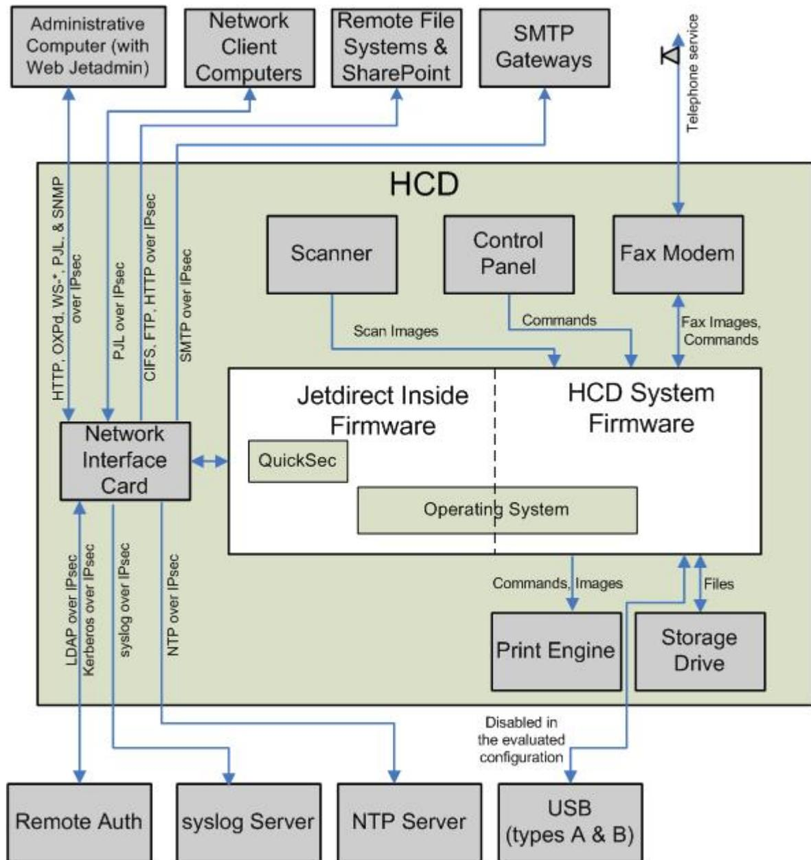
**Figure 1: HCD physical diagram**
