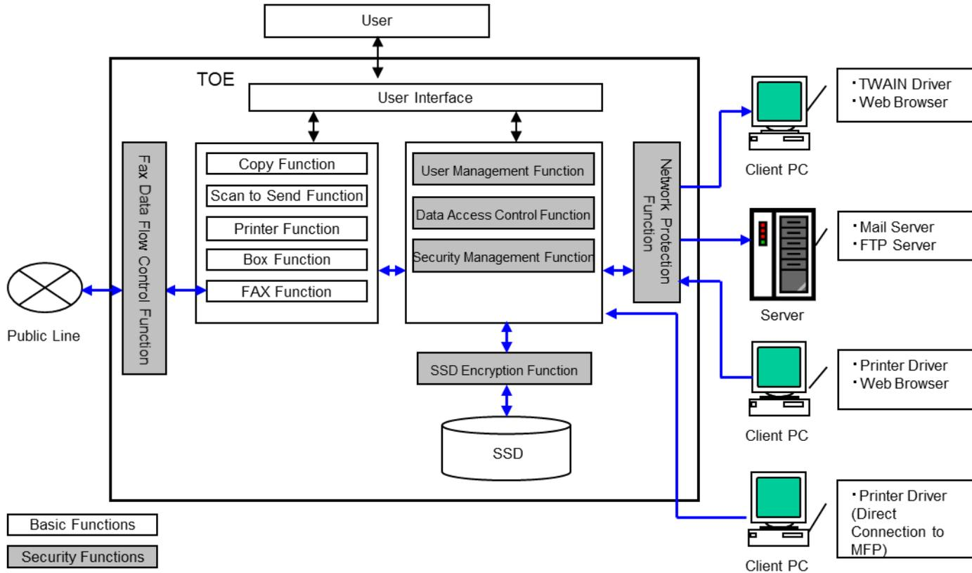
Please see section 1.4.3 in the [ST] for a more detailed description of the functionality shown in the diagram. There is no interface for any user or administrator to directly interact with the TOE operating system, all interactions must be made via one of the standard application functions or the hardware interfaces of the TOE.
