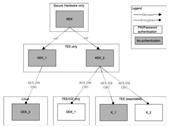
Figure 3 - Key Management Diagram for Full Disk Encryption
