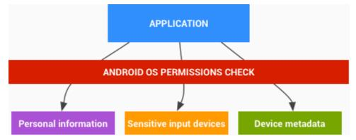
Figure 4 - Access to sensitive user data, input devices and metadata is available only through protected APIs that will perform permission checks
