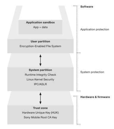
Figure 1 - The Android architecture used by Xperia
